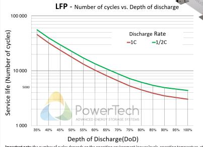
**Important note**: the number of cycles depends on the operating environment (power levels, operating temperature, etc.). These data have been obtained from laboratory tests in a controlled environment.
